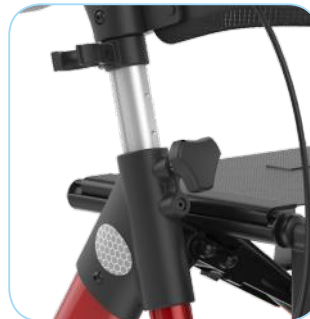
Flattened handle height adjustment tubes.
